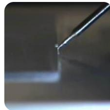
Notice the uniformity of line width and uniform starts and ends. GPD Global pump technology eliminates “snake heads” that are common with other technologies.
