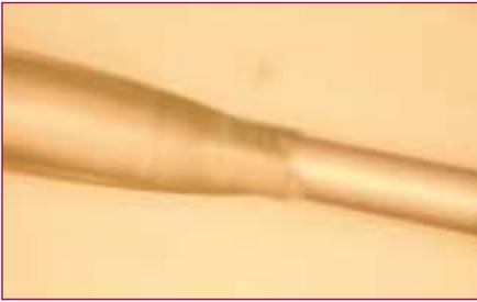
Figure 2. Illustration displays a fiber with the buffer material removed, and the glass cladding and core exposed.
